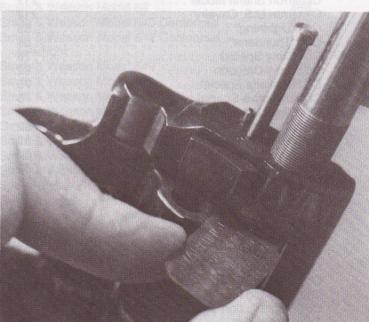
When replacing the barrel, remember that the end with the longer threaded section goes toward the rear. Insert the gauge supplied with the gun between the rear face of the barrel and the front of the cylinder, and turn the barrel until it is snug, but don't over-tighten it. Leave the gauge in place while installing the barrel shroud. If the original gauge is not with the gun, any .006-inch leaf (feeler) gauge will work.
