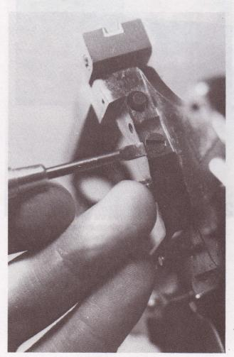
**26.** Drifting out the small roll pin at the upper rear of the frame will release the firing pin and its spring for removal toward the rear. Drifting out the roll pin at the top of the frame, above the cylinder opening, will partially free the rear sight.
