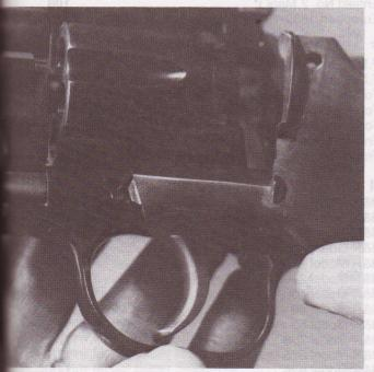
**3.** When replacing the sideplate, remember that the lip at its front edge must be put in first, then the rear of the plate moved inward.
