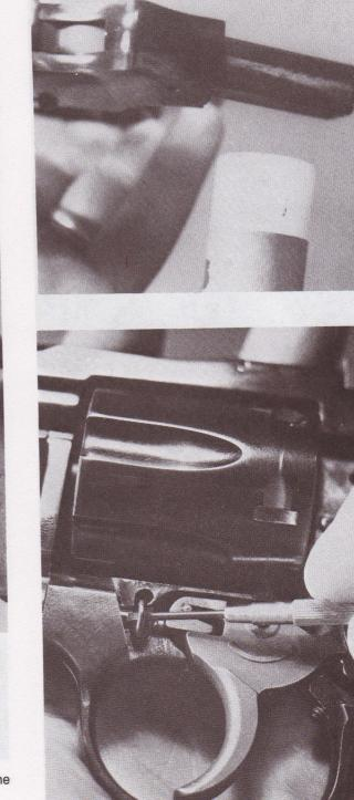
7. Use a small screwdriver to lift out and remove the U-shaped crane retainer toward the left.
