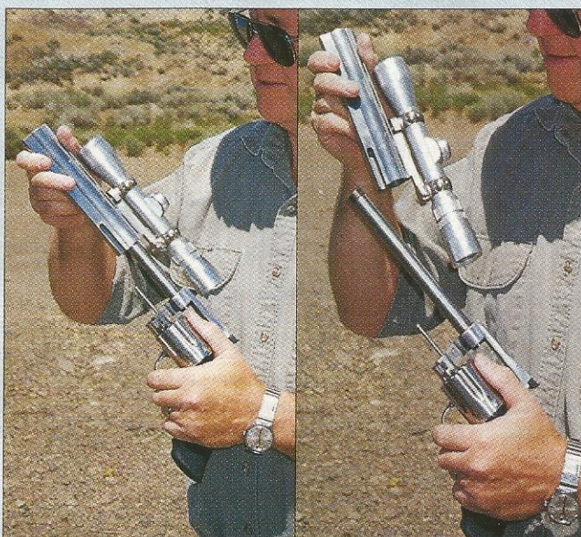
Next, pull the shroud forward and clear of the barrel.
