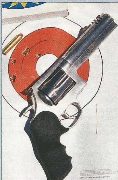
With the author employing the 4-inch version from a sitting position, the Dan Wesson Super Mag punched five-shot, 2½-inch groups at 25 yards (left) with 250-grain ammo. At 50 yards from a sandbagged rest using the 8-inch scoped barrel, his best effort was a 1½-inch three-shot group (above) using the 300-grain factory loads.
