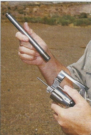
The first step in switching barrels is to remove the front barrel nut with the Dan Wesson tool.
