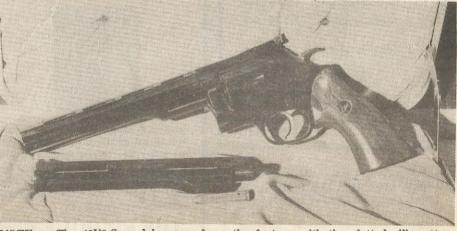
NOTE: The 40V8-S model comes from the factory with the slotted silhouette barrel shown above installed on the gun instead of the non-slotted shroud shown on the gun above. A extra 8-inch, non-ported barrel only comes with each gun.
