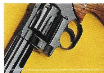
Unique placement of the cylinder latch close to the barrel-cylinder gap stabilizes the cylinder in its alignment, aiding accuracy, and eliminates fragile parts, making the gun unusually rugged.
